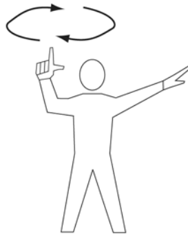
Circular motion of right hand at head level with left arm pointing to engine. START ENGINE
